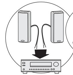
Note: Make sure to connect the + terminal on the speaker to the + terminal on the amplifier and connect the - terminal on the speaker to the - terminal on the amplifier.
